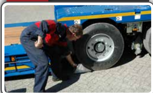
37 Remove wheel wedges
