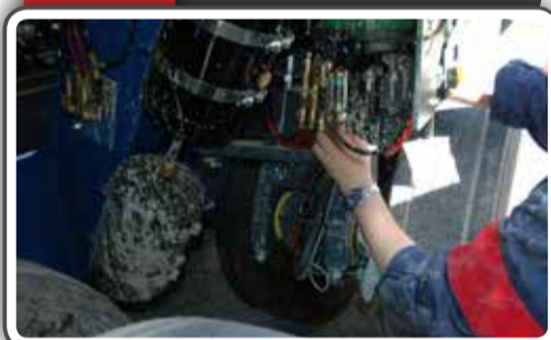
30 Replace hose bundle behind axle knee
