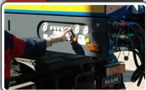
38 Raise axle bogie up to ride height
