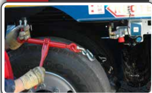
34 Remove chain spanner
