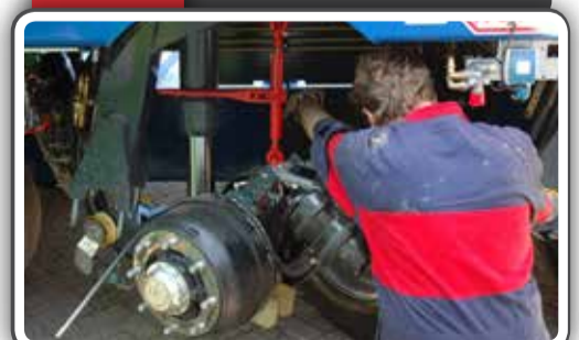
20 Place new inside wheel
