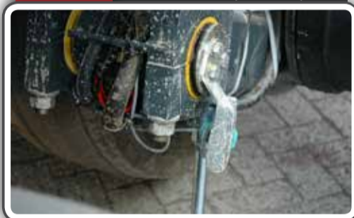
29 Tighten back nuts axle knee(250Nm)
