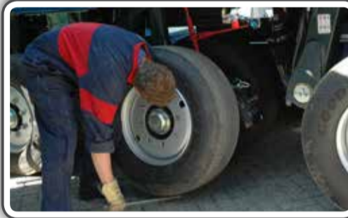
31 Place outside wheel on axle
