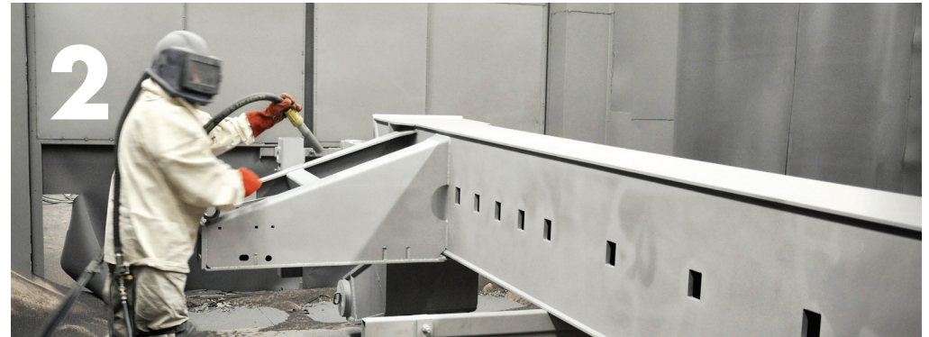
The entire chassis is blasted with corundum, an extremely hard aluminium oxide that is used to remove rust and dirt. When the chassis is as clean as a whistle, the surface is ready to be sprayed with layer of metal coating.
