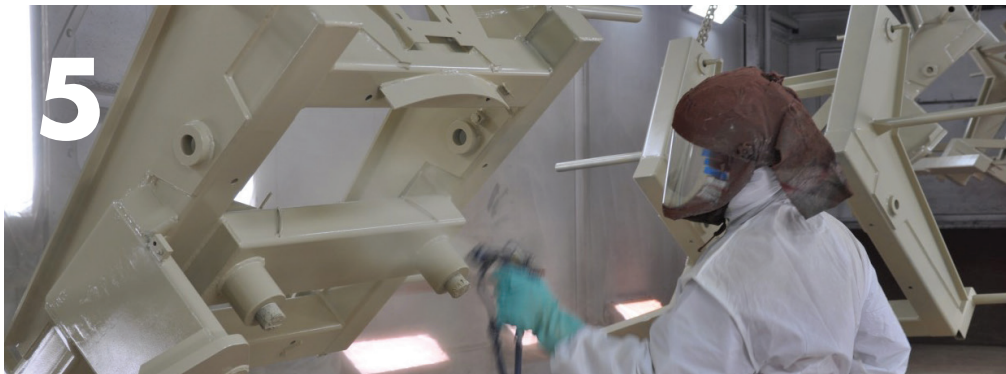
After the anti-corrosion treatment follows the application of two layers of PUR primer, the adhesive coat and corrosion-prevention for the paint.
