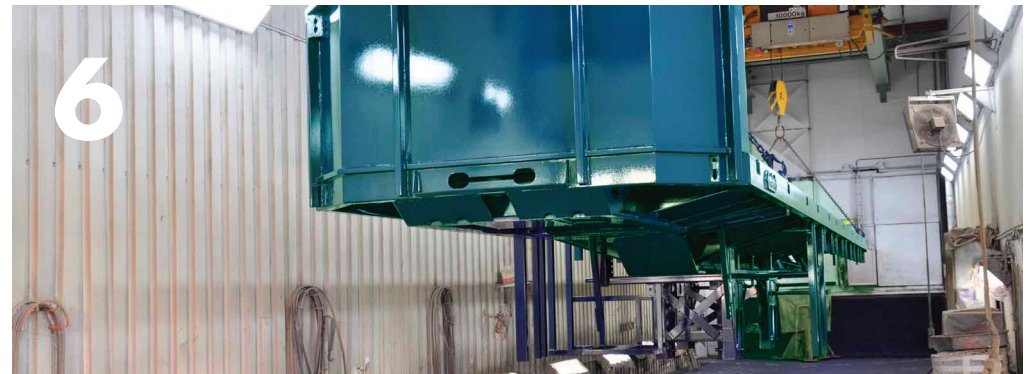
The trailer is sprayed – wet on wet in two coats – with high-quality polyurethane (PU) paint that provides an extremely hard, durable gloss and excellent scratch resistance. The coating will keep the trailer looking good for the next 10 to 12 years.
